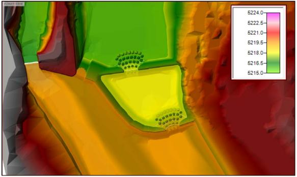
Figure 28. Water surface elevation at river flows of 475 cfs, Fruitland-Cambridge diversion of 145 cfs, and 100 cfs through radial gates adjacent to canal inlet.
