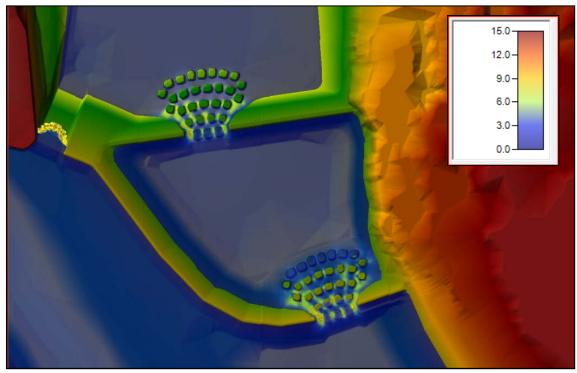
Figure 27. Water velocity distribution (ft/sec) at river flows of 475 cfs, Fruitland-Cambridge diversion of 145 cfs, and 100 cfs through radial gates adjacent to canal inlet.
