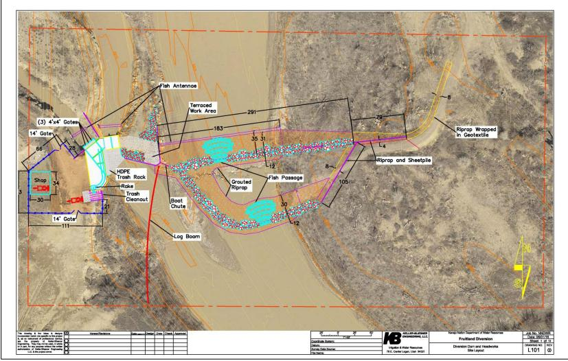
Figure 5. Proposed two-step diversion dam, fish and boat passage, and headworks (NNDWR 2016).
